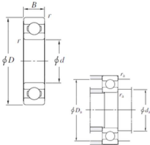
6021 Bearing 2D drawings and 3D CAD models
